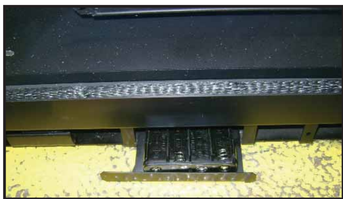
Figure 2.5 Battery Tray Pulled Out
